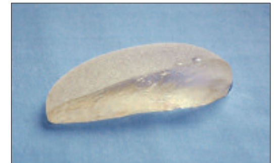
Photograph of a cohesive silicone gel implant cut in half - the silicone retains its shape due to increased cross-linking of the silicone molecules
